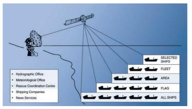
Basic concept of the Inmarsat Enhanced Group Calling System (the shaded area indicates functions of the SafetyNet<sup>™</sup> Service)
